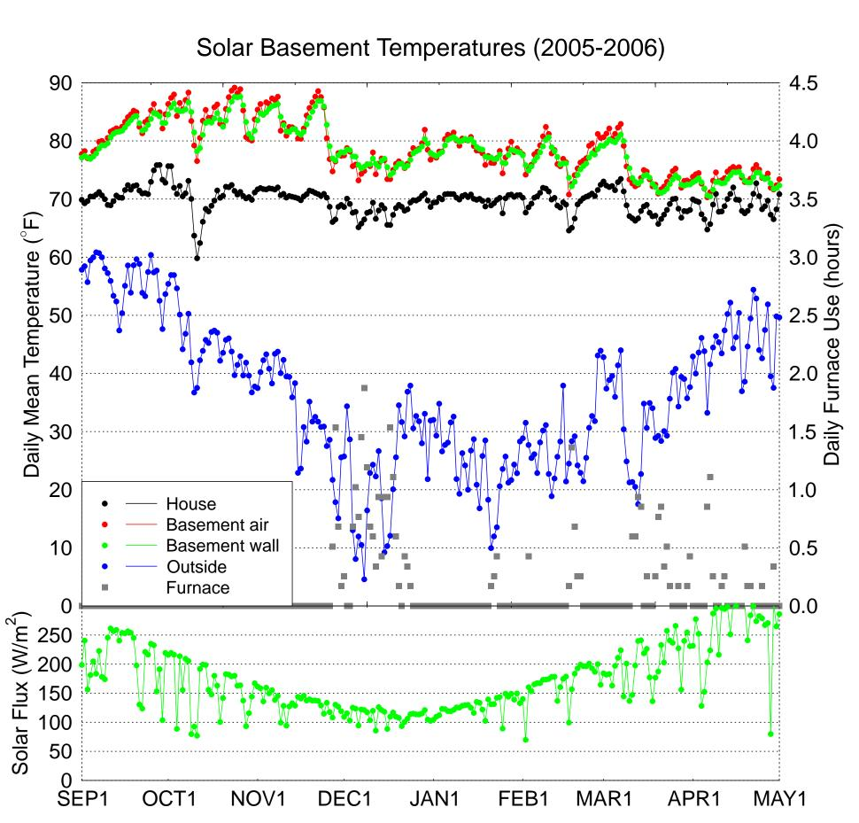
The graph above shows the observed daily average temperatures and solar flux for the last heating season. The gray squares (and righthand axis) show how long the backup propane furnace ran each day.
